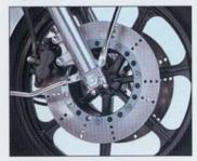
Updated dual front disc brakes feature new twin opposed-piston calipers and new pads. Updated rear brake linkage and a new twin opposed-piston caliper add dependable braking performance.
