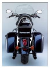
\* In addition to the windscreen and panniers from the VN1500L, the new Classic Tourer receives a number of new features designed to increase passenger comfort. These include the addition of a backrest and passenger grab rails. (Photos 3-5)
