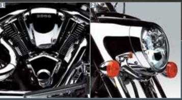
Category-shattering performance from a liquid-cooled 2,053 cm³ V-Twin engine pumping out an awesome spread of torque across the rpm range. High-tech features include 4-valve OHV heads, lightweight slipper pistons sliding in plated alloy cylinders and a sophisticated, electronic fuel injection system featuring huge 46 mm throttle bodies.
