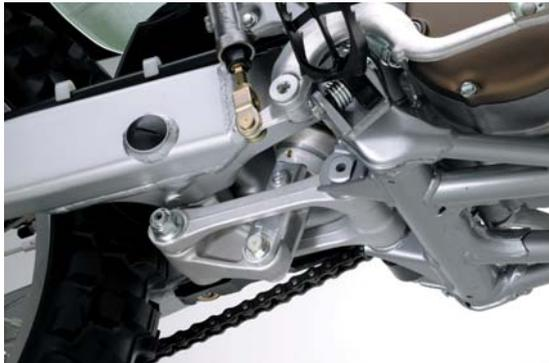
'03 chassis in which the link pivoted on the frame, in the new system, a newly designed link pivots on the swingarm. The advantages are twofold: first, the brunt of the suspension loads are now absorbed by the swingarm, allowing a lighter frame construction. The second benefit is that the shock absorber now moves in an outward arc as it compresses, rather than moving out and back in. This smoother, more stable action significantly improves traction.
