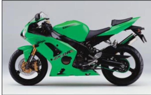
**Lightweight aluminium frame with central Ram Air duct**
