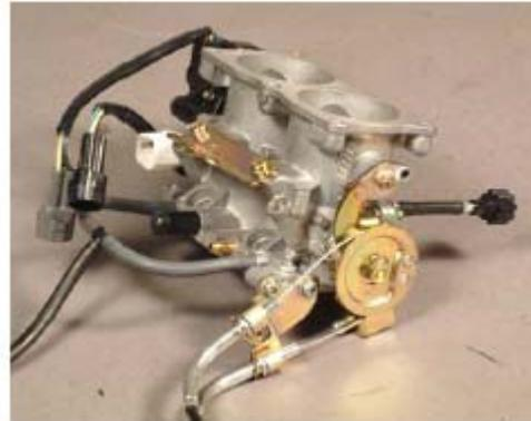
■ High atomising fuel injectors produce a fine fuel mist for better combustion, fuel consumption and low emissions.
