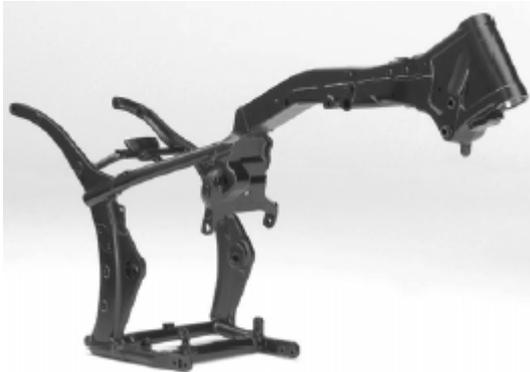
■ A cast steering head and one-piece cast frame rails at the swingarm pivot require fewer welds and parts for a clean appearance.
