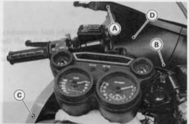
A. Screws (Left and Right) B. Screw (Center) C. Screws (Left and Right) D. Upper Fairing
